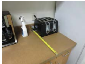
Access specialist verifies work surface maximum height of 34” AFF, unobstructed side maximum high reach of 48” AFF and maximum depth of 10” to appliances’ operable parts. A maximum depth of 24” is allowed when the side maximum high reach is 46” AFF.
